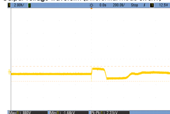
Output voltage waveform (Common mode 0.88 kV)
